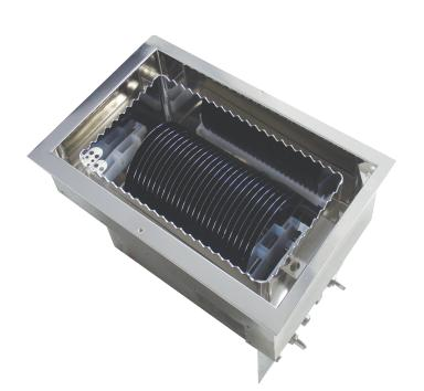
JST's Ambient Filtration bath continuously filters process chemicals in a laminar flow direction from the bottom of the bath upward over a four sided weir. The bath is designed to filter sub-micron particles and reduce chemical consumption.
