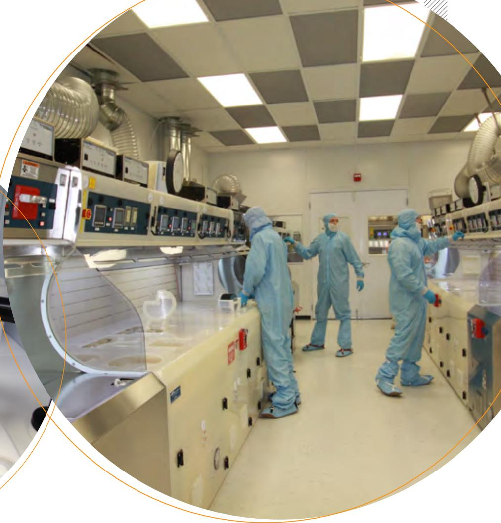
Whether for compound semiconductor, nanotechnology, Micro-Electro-Mechanical Systems (MEMS), biophotonics, biomedical electronics, or creating solar power alternatives to traditional silicon wafer construction, much of the advanced research done in labs today requires microfabrication operations. This typically includes wet processing equipment for metal lift-off, stripping, etching, plating/coating, cleaning, and de-bonding.
