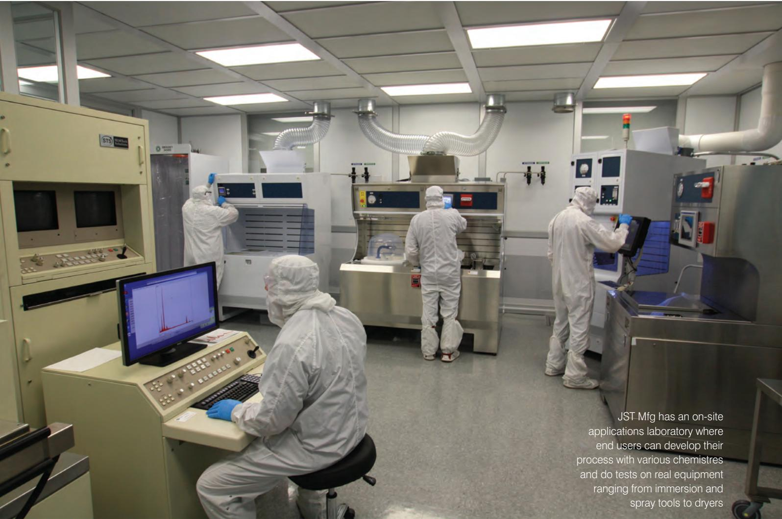
JST Mfg has an on-site applications laboratory where end users can develop their process with various chemistries and do tests on real equipment ranging from immersion and spray tools to dryers
