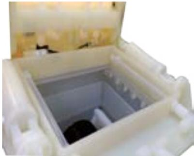
JST's Combination Rinse and STG Dryer is capable of Quick Dump Rinsing (QDR) and IPA vapor drying substrates in a single chamber eliminating air contact. The STG Dryer is able to dry both hydrophobic and hydrophilic wafers with low particle adders (<10 @0.16um). It is also compatible with drying wafers with exposed resist without affecting the resist.
