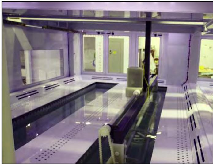
Wet processing chamber for cleaning and etching.
