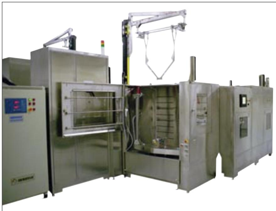
Optics up to 300 pounds are loaded onto the JST Automated Optics Cleaner where they are cleaned, rinsed and dried prior to being installed in the NIF facility.
