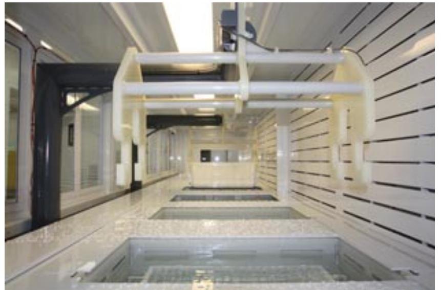
Racks and fixtures need to be designed to safely handle parts and the fixtures themselves must be designed to withstand the chemicals involved.
