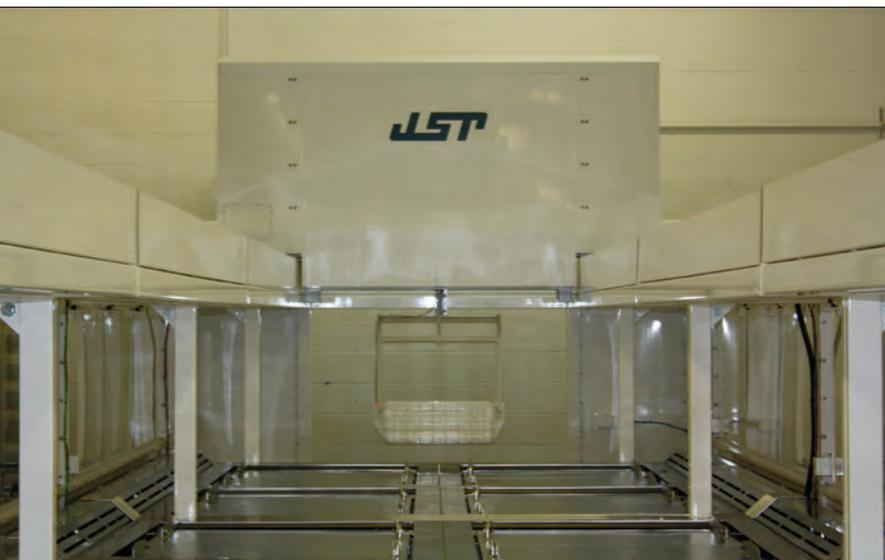
or when products are temperature sensitive. In an N2 blowoff dryer approach, nitrogen is blown into the drying chamber through high pressure air knives. The moisture is blown off the product and down into the plenum where it is evacuated in the exhaust stream. Although the process is initially lower in cost, it uses a lot of nitrogen, may not totally dry product, and does not work with geometries that retain moisture when removed, including those with blind holes.
