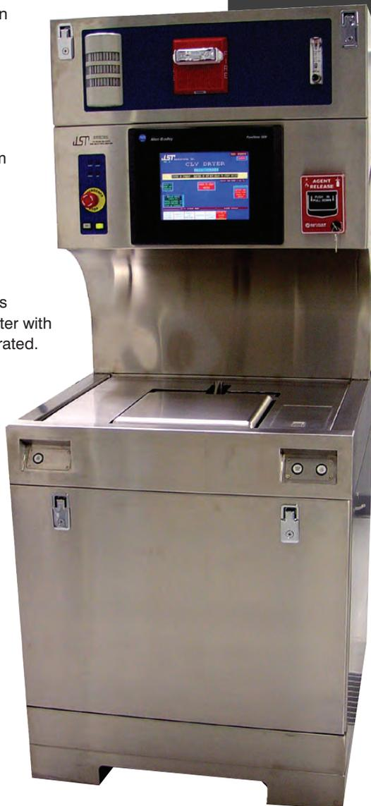
The closed loop system allows fresh IPA vapor to rinse the surface to be dried, penetrating the surface areas and absorbing the moisture. A low pressure vacuum pulls any remaining moisture from the sealed chamber and away from the product being dried.
