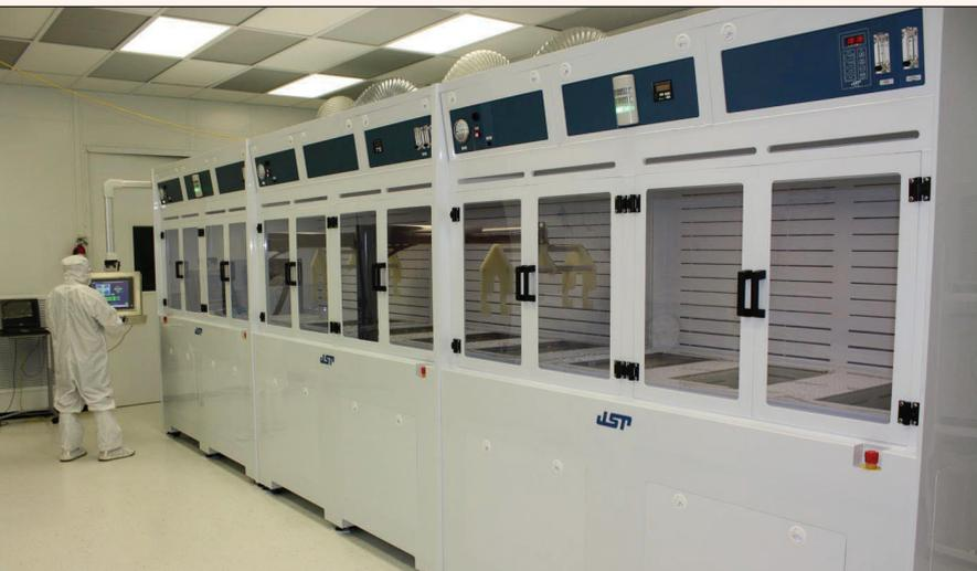
entailed building a cleaning line 138 ft. in length and incorporating multiple gantry robots.
